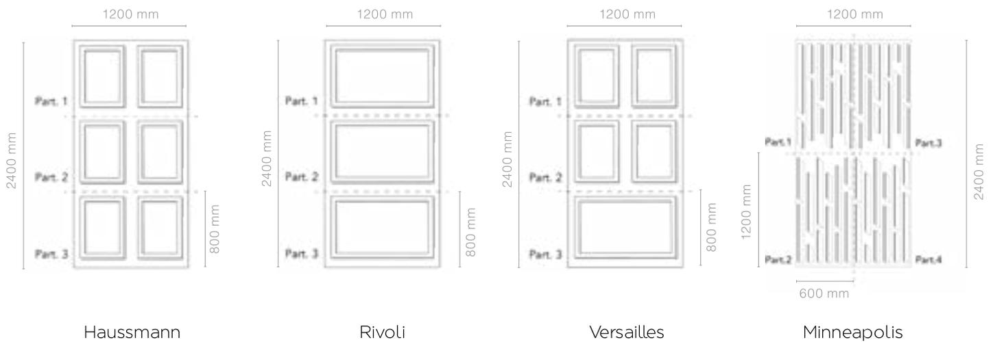
*Designed and delivered as a kit of 3 or 4 panels, 2.88m<sup>2</sup>*
