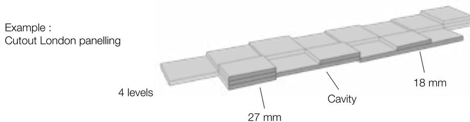
3D structures with invisible cavities to optimise acoustic absorption
