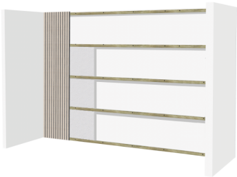
Rock wool : width 600 mm / thickness 20 mm / density +/- 100kg/m3
